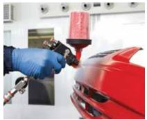
With the 1.2mm and 1.3mm atomizing heads, you can go from start to finish on bumpers: primer, sealer, basecoat and clearcoat.
